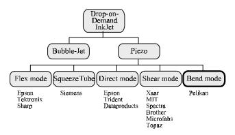
Figure 1: Inkjet printhead technologies
