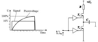
Figure 5: Drive electronics for a bend mode actuator printhead
