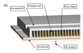
Figure 2: Major parts of an bend mode actuator printhead (A) before assembly (B) assembled
