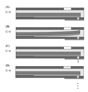
Figure 6: Droplet ejection process
