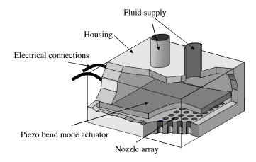
Figure 9: Sprayer based on a bend mode actuator
