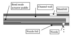
Figure 3. Cross section of a bend mode actuator piezo printhead
