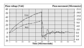
Figure 4: Voltage and movement of the piezo
